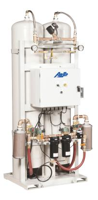
AirSep Alpha Series Oxygen Generators produce from 20 to 5,500 cubic feet of oxygen per hour at up to 95% oxygen concentration. When electricity and a source of compressed air is supplied, these dependable machines can provide oxygen for practically any application.
